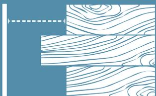
When you arrive at the end of the Wall, measure with a ruler the distance from the last tile in the Wall and mark the tile you will cut.
