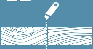
To collocate the tile, mark with a pencil the cut line. Collocate on the line, a square or metallic ruler and pass softly the cutter over the mark once.
